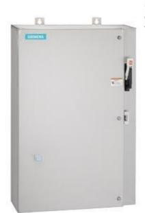
Non-reversing motor starter Size 0 Three phase full voltage Amb compensate bimetal OLrelay Contactor amp rating 18Amp 240VAC 50HZ / 277VAC 60HZ coil Combination type 30Amp fusible disconnect 30 Amp /600V fuse clip Encl NEMA type 4X 316 S-steel Water/dust tight non-corrosive Extra-wide enclosure
