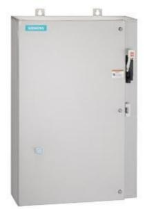
Non-reversing motor starter Size 0 Three phase full voltage Amb compensate bimetal OLrelay Contactor amp rating 18Amp 240VAC 50HZ / 277VAC 60HZ coil Combination type 30Amp fusible disconnect 30 Amp /600V fuse clip Encl NEMA type 4X 316 S-steel Water/dust tight non-corrosive Extra-wide enclosure
