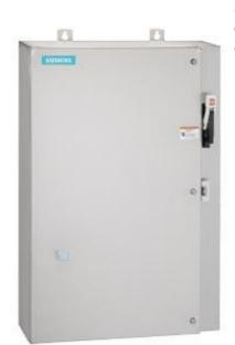
Non-reversing motor starter Size 0 Three phase full voltage Amb compensate bimetal OLrelay Contactor amp rating 18Amp 240VAC 50HZ / 277VAC 60HZ coil Combination type 30Amp non-fusible disconnect Encl NEMA type 4X 316 S-steel Water/dust tight non-corrosive Extra-wide enclosure
