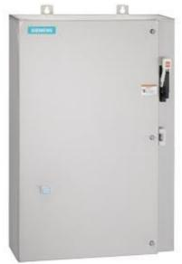
Non-reversing motor starter Size 0 Three phase full voltage Amb compensate bimetal OLrelay Contactor amp rating 18Amp 240VAC 50HZ / 277VAC 60HZ coil Combination type 30Amp non-fusible disconnect Encl NEMA type 4X 316 S-steel Water/dust tight non-corrosive Extra-wide enclosure
