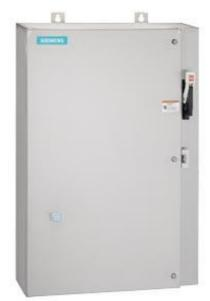
Non-reversing motor starter Size 0 Three phase full voltage Amb compensate bimetal OLrelay Contactor amp rating 18Amp 24Vdc coil Combination type 30Amp non-fusible disconnect Encl NEMA type 4X 316 S-steel Water/dust tight non-corrosive Extra-wide enclosure
