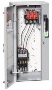
Non-reversing motor starter Size 0 Three phase full voltage Amb compensate bimetal OLrelay Contactor amp rating 18Amp 220-240/440-480VAC 60HZ coil Combination type 30Amp non-fusible disconnect Enclosure NEMA type 1 Indoor general purpose use Standard width enclosure
