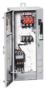
Non-reversing motor starter Size 0 Three phase full voltage Amb compensate bimetal OLrelay Contactor amp rating 18Amp 110-120/220-240VAC 60HZ coil Combination type 30Amp fusible disconnect 30Amp / 250V fuse clip Enclosure NEMA type 4/12 Water/dust tight weather proof Standard width enclosure
