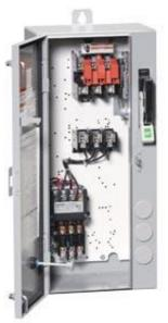
Non-reversing motor starter Size 0 Three phase full voltage Amb compensate bimetal OLrelay Contactor amp rating 18Amp Combination type 30Amp fusible disconnect 30Amp / 250V fuse clip Enclosure NEMA type 4/12 Water/dust tight weather proof Standard width enclosure
