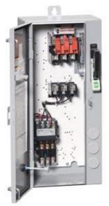
Non-reversing motor starter Size 0 Three phase full voltage Amb compensate bimetal OLrelay Contactor amp rating 18Amp 208VAC 60HZ coil Combination type 30Amp fusible disconnect 30Amp / 250V fuse clip Enclosure NEMA type 4/12 Water/dust tight weather proof Standard width enclosure
