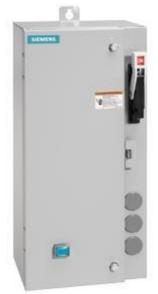
Non-reversing motor starter Size 0 Three phase full voltage Amb compensate bimetal OLrelay Contactor amp rating 18Amp 208VAC 60HZ coil Combination type 30Amp non-fusible disconnect Enclosure NEMA type 4/12 Water/dust tight weather proof Standard width enclosure
