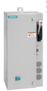
Non-reversing motor starter Size 0 Three phase full voltage Amb compensate bimetal OLrelay Contactor amp rating 18Amp 550/575-600 50/60HZ coil Combination type 30Amp non-fusible disconnect Enclosure NEMA type 4/12 Water/dust tight weather proof Standard width enclosure
