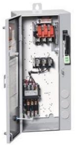
Non-reversing motor starter, Size 0, Three phase full voltage, Amb compensate bimetal OLrelay Contactor amp rating 18Amp 110V 50HZ / 120V 60HZ coil, Combination type, 30Amp fusible disconnect 30 Amp /600V fuse clip, Enclosure NEMA type 4/12, Water/dust tight for outdoors, Standard width enclosure
