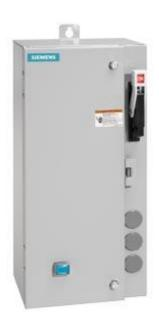
Non-reversing motor starter Size 0 Three phase full voltage Amb compensate bimetal OLrelay Contactor amp rating 18Amp 110VAC 50HZ / 120VAC 60HZ coil Combination type 30Amp non-fusible disconnect Enclosure NEMA type 4/12 Water/dust tight weather proof Standard width enclosure
