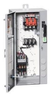
Non-reversing motor starter Size 0 Three phase full voltage Amb compensate bimetal OLrelay Contactor amp rating 18Amp Combination type 30Amp fusible disconnect 30Amp / 250V fuse clip Enclosure NEMA type 4/12 Water/dust tight weather proof Standard width enclosure
