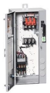
Non-reversing motor starter Size 0 Three phase full voltage Amb compensate bimetal OLrelay Contactor amp rating 18Amp Combination type 30Amp fusible disconnect 30 Amp /600V fuse clip Enclosure NEMA type 4/12 Water/dust tight weather proof Standard width enclosure
