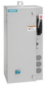
Non-reversing motor starter Size 0 Three phase full voltage Amb compensate bimetal OLrelay Contactor amp rating 18Amp 190-220/220-240V 50/60HZ coil Combination type 30Amp non-fusible disconnect Enclosure NEMA type 4/12 Water/dust tight weather proof Standard width enclosure
