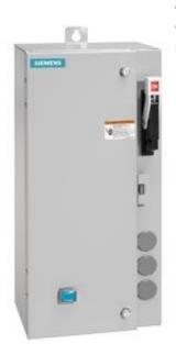
Non-reversing motor starter Size 0 Three phase full voltage Amb compensate bimetal OLrelay Contactor amp rating 18Amp 380-440/440-480V 50/60HZ coil Combination type 30Amp non-fusible disconnect Enclosure NEMA type 4/12 Water/dust tight weather proof Standard width enclosure
