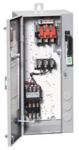
Non-reversing motor starter Size 0 Three phase full voltage Amb compensate bimetal OLrelay Contactor amp rating 18Amp 24VAC 50-60HZ coil Combination type 30Amp fusible disconnect 30Amp / 250V fuse clip Enclosure NEMA type 4/12 Water/dust tight weather proof Standard width enclosure
