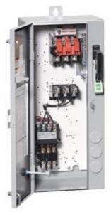
Non-reversing motor starter Size 0 Three phase full voltage Amb compensate bimetal OLrelay Contactor amp rating 18Amp 240VAC 50HZ / 277VAC 60HZ coil Combination type 30Amp fusible disconnect 30 Amp /600V fuse clip Enclosure NEMA type 4/12 Water/dust tight weather proof Standard width enclosure
