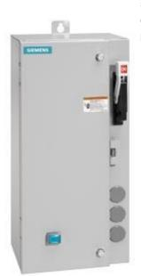
Non-reversing motor starter Size 0 Three phase full voltage Amb compensate bimetal OLrelay Contactor amp rating 18Amp 240VAC 50HZ / 277VAC 60HZ coil Combination type 30Amp non-fusible disconnect Enclosure NEMA type 4/12 Water/dust tight weather proof Standard width enclosure
