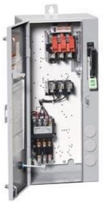
Non-reversing motor starter Size 0 Three phase full voltage Amb compensate bimetal OLrelay Contactor amp rating 18Amp 24Vdc coil Combination type 30Amp fusible disconnect 30Amp / 250V fuse clip Enclosure NEMA type 4/12 Water/dust tight weather proof Standard width enclosure
