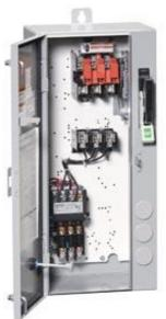
Non-reversing motor starter Size 0 Three phase full voltage Amb compensate bimetal OLrelay Contactor amp rating 18Amp 24Vdc coil Combination type 30Amp fusible disconnect 30 Amp /600V fuse clip Enclosure NEMA type 4/12 Water/dust tight weather proof Standard width enclosure
