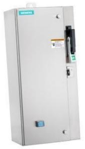
Non-reversing motor starter Size 0 Three phase full voltage Amb compensate bimetal OLrelay Contactor amp rating 18Amp Combination type 30Amp fusible disconnect 30 Amp /600V fuse clip Encl NEMA type 4X 304 S-steel Water/dust tight non-corrosive Standard width enclosure
