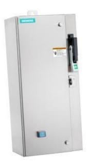
Non-reversing motor starter Size 0 Three phase full voltage Amb compensate bimetal OLrelay Contactor amp rating 18Amp 110-120/220-240VAC 60HZ coil Combination type 30Amp non-fusible disconnect Encl NEMA type 4X 304 S-steel Water/dust tight non-corrosive Standard width enclosure
