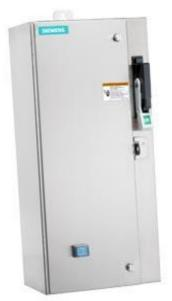
Non-reversing motor starter Size 0 Three phase full voltage Amb compensate bimetal OLrelay Contactor amp rating 18Amp Combination type 30Amp fusible disconnect 30Amp / 250V fuse clip Encl NEMA type 4X 304 S-steel Water/dust tight non-corrosive Standard width enclosure
