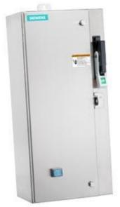
Non-reversing motor starter Size 0 Three phase full voltage Amb compensate bimetal OLrelay Contactor amp rating 18Amp 220-240/440-480VAC 60HZ coil Combination type 30Amp non-fusible disconnect Encl NEMA type 4X 304 S-steel Water/dust tight non-corrosive Standard width enclosure
