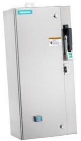
Non-reversing motor starter Size 0 Three phase full voltage Amb compensate bimetal OLrelay Contactor amp rating 18Amp 208VAC 60HZ coil Combination type 30Amp fusible disconnect 30Amp / 250V fuse clip Encl NEMA type 4X 304 S-steel Water/dust tight non-corrosive Standard width enclosure
