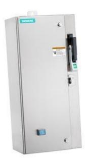
Non-reversing motor starter Size 0 Three phase full voltage Amb compensate bimetal OLrelay Contactor amp rating 18Amp 208VAC 60HZ coil Combination type 30Amp non-fusible disconnect Encl NEMA type 4X 304 S-steel Water/dust tight non-corrosive Standard width enclosure
