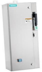
Non-reversing motor starter Size 0 Three phase full voltage Amb compensate bimetal OLrelay Contactor amp rating 18Amp Combination type 30Amp non-fusible disconnect Encl NEMA type 4X 304 S-steel Water/dust tight non-corrosive Standard width enclosure
