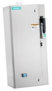
Non-reversing motor starter Size 0 Three phase full voltage Amb compensate bimetal OLrelay Contactor amp rating 18Amp 380-440/440-480V 50/60HZ coil Combination type 30Amp non-fusible disconnect Encl NEMA type 4X 304 S-steel Water/dust tight non-corrosive Standard width enclosure
