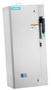
Non-reversing motor starter Size 0 Three phase full voltage Amb compensate bimetal OLrelay Contactor amp rating 18Amp 24VAC 50-60HZ coil Combination type 30Amp fusible disconnect 30 Amp /600V fuse clip Encl NEMA type 4X 304 S-steel Water/dust tight noncorrosive Standard width enclosure
