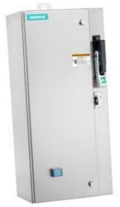
Non-reversing motor starter Size 0 Three phase full voltage Amb compensate bimetal OLrelay Contactor amp rating 18Amp 24VAC 50-60HZ coil Combination type 30Amp non-fusible disconnect Encl NEMA type 4X 304 S-steel Water/dust tight non-corrosive Standard width enclosure
