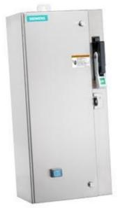
Non-reversing motor starter Size 0 Three phase full voltage Amb compensate bimetal OLrelay Contactor amp rating 18Amp 240VAC 50HZ / 277VAC 60HZ coil Combination type 30Amp non-fusible disconnect Encl NEMA type 4X 304 S-steel Water/dust tight non-corrosive Standard width enclosure
