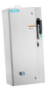
Non-reversing motor starter Size 0 Three phase full voltage Amb compensate bimetal OLrelay Contactor amp rating 18Amp 24Vdc coil Combination type 30Amp fusible disconnect 30 Amp /600V fuse clip Encl NEMA type 4X 304 S-steel Water/dust tight non-corrosive Standard width enclosure
