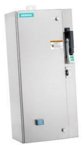
Non-reversing motor starter Size 0 Three phase full voltage Amb compensate bimetal OLrelay Contactor amp rating 18Amp 24Vdc coil Combination type 30Amp non-fusible disconnect Encl NEMA type 4X 304 S-steel Water/dust tight non-corrosive Standard width enclosure
