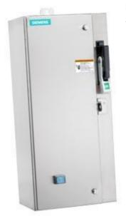
Non-reversing motor starter Size 0 Three phase full voltage Amb compensate bimetal OLrelay Contactor amp rating 18Amp Combination type 30Amp fusible disconnect 30Amp / 250V fuse clip Encl NEMA type 4X 316 S-steel Water/dust tight non-corrosive Standard width enclosure
