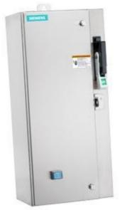
Non-reversing motor starter Size 0 Three phase full voltage Amb compensate bimetal OLrelay Contactor amp rating 18Amp Combination type 30Amp fusible disconnect 30 Amp /600V fuse clip Encl NEMA type 4X 316 S-steel Water/dust tight non-corrosive Standard width enclosure
