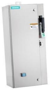
Non-reversing motor starter Size 0 Three phase full voltage Amb compensate bimetal OLrelay Contactor amp rating 18Amp 208VAC 60HZ coil Combination type 30Amp fusible disconnect 30Amp / 250V fuse clip Encl NEMA type 4X 316 S-steel Water/dust tight non-corrosive Standard width enclosure
