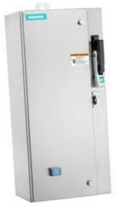
Non-reversing motor starter Size 0 Three phase full voltage Amb compensate bimetal OLrelay Contactor amp rating 18Amp 208VAC 60HZ coil Combination type 30Amp fusible disconnect 30 Amp /600V fuse clip Encl NEMA type 4X 316 S-steel Water/dust tight non-corrosive Standard width enclosure
