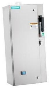
Non-reversing motor starter Size 0 Three phase full voltage Amb compensate bimetal OLrelay Contactor amp rating 18Amp 110VAC 50HZ / 120VAC 60HZ coil Combination type 30Amp fusible disconnect 30 Amp /600V fuse clip Encl NEMA type 4X 316 S-steel Water/dust tight non-corrosive Standard width enclosure
