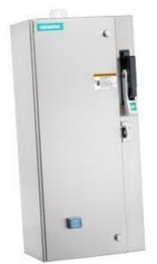
Non-reversing motor starter Size 0 Three phase full voltage Amb compensate bimetal OLrelay Contactor amp rating 18Amp Combination type 30Amp non-fusible disconnect Encl NEMA type 4X 316 S-steel Water/dust tight non-corrosive Standard width enclosure
