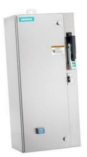
Non-reversing motor starter Size 0 Three phase full voltage Amb compensate bimetal OLrelay Contactor amp rating 18Amp Combination type 30Amp fusible disconnect 30Amp / 250V fuse clip Encl NEMA type 4X 316 S-steel Water/dust tight non-corrosive Standard width enclosure
