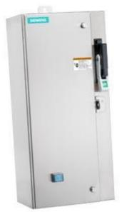
Non-reversing motor starter Size 0 Three phase full voltage Amb compensate bimetal OLrelay Contactor amp rating 18Amp Combination type 30Amp non-fusible disconnect Encl NEMA type 4X 316 S-steel Water/dust tight non-corrosive Standard width enclosure
