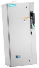
Non-reversing motor starter Size 0 Three phase full voltage Amb compensate bimetal OLrelay Contactor amp rating 18Amp 24VAC 50-60HZ coil Combination type 30Amp fusible disconnect 30 Amp /600V fuse clip Encl NEMA type 4X 316 S-steel Water/dust tight non-corrosive Standard width enclosure
