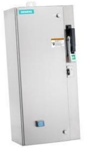
Non-reversing motor starter Size 0 Three phase full voltage Amb compensate bimetal OLrelay Contactor amp rating 18Amp 24VAC 50-60HZ coil Combination type 30Amp non-fusible disconnect Encl NEMA type 4X 316 S-steel Water/dust tight non-corrosive Standard width enclosure
