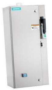
Non-reversing motor starter Size 0 Three phase full voltage Amb compensate bimetal OLrelay Contactor amp rating 18Amp 240VAC 50HZ / 277VAC 60HZ coil Combination type 30Amp fusible disconnect 30 Amp /600V fuse clip Encl NEMA type 4X 316 S-steel Water/dust tight non-corrosive Standard width enclosure
