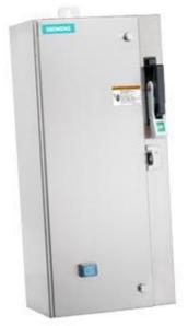
Non-reversing motor starter Size 0 Three phase full voltage Amb compensate bimetal OLrelay Contactor amp rating 18Amp 240VAC 50HZ / 277VAC 60HZ coil Combination type 30Amp non-fusible disconnect Encl NEMA type 4X 316 S-steel Water/dust tight non-corrosive Standard width enclosure
