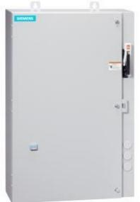
Non-reversing motor starter Size 0 Three phase full voltage Solidstate overload relay OLRelay amp range 0.25-1A 24Vdc coil Combination type 30Amp fusible disconnect 30 Amp /600V fuse clip Encl NEMA type 4X 304 S-steel Water/dust tight non-corrosive Extrawide enclosure
