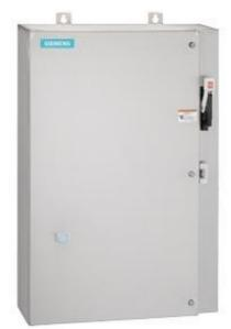
Non-reversing motor starter Size 0 Three phase full voltage Solidstate overload relay OLRelay amp range 0.25-1A Combination type 30Amp fusible disconnect 30 Amp /600V fuse clip Encl NEMA type 4X 316 S-steel Water/dust tight non-corrosive Extra-wide enclosure
