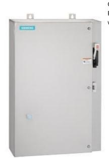
Non-reversing motor starter Size 0 Three phase full voltage Solidstate overload relay OLRelay amp range 0.25-1A 208VAC 60HZ coil Combination type 30Amp fusible disconnect 30Amp / 250V fuse clip Encl NEMA type 4X 316 S-steel Water/dust tight non-corrosive Extrawide enclosure
